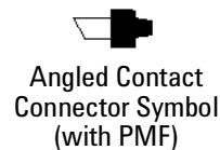
Figure 4 Angled Contact Connector Symbols
